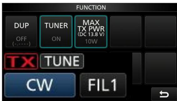
Enter the function menu of the transmitter, as shown in the figure, the [TUNER] option turns white to indicate that it is available.
