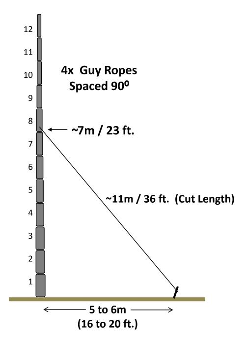
Attach 3 (preferably 4) guy lines to the pole above segment number 7 (height = 7m). We recommend a guying distance from the pole of 5 to 6m. This results in a guy line Length of approx. 11m. You will need 4x 11m = 44m of 2mm Kevlar rope. We recommend purchasing one roll (50m) of Kevlar rope and cutting it into 4 pieces, each 12m long. NOTE: 1m = 3.3 ft.
