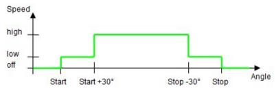
The rotators from Yaesu $^{TM}$  allow the speed-control in 4 stages:1 - 2 - 3 - 4, where 1 is the lowest speed and 4 is the highest speed
