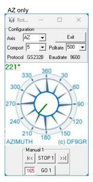
The green pointers and numbers show the current position of the rotators. Targets can be put at the red numbers. You can control the rotators for Azimuth and Elevation separately or together. Click the GO-buttons or click on any point of the graphics to start the rotation and click the STOP-buttons to stop rotation.
