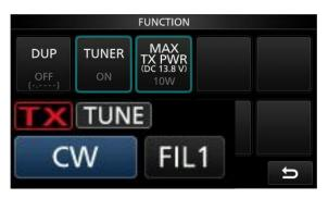
Enter the function menu of the transmitter, as shown in the figure, the [TUNER] option turns white to indicate that it is available.
