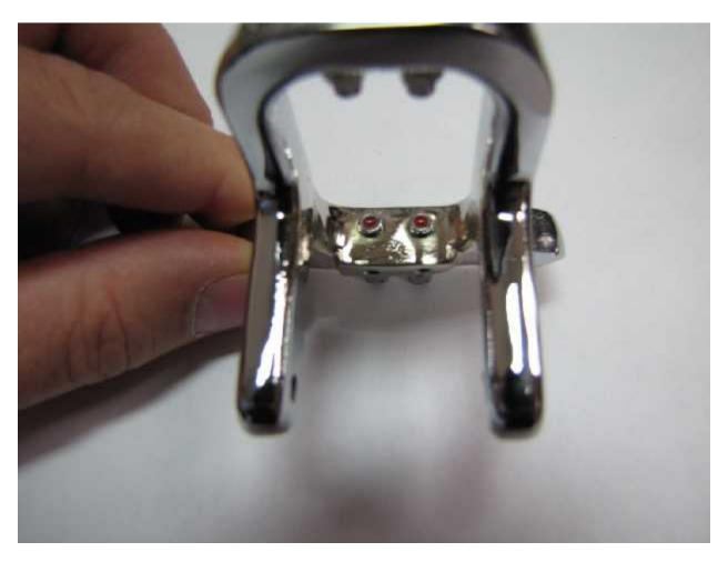
The trunion pins themselves are mounted through the lever(s) of the key. When you touch the finger paddles to send code, the trunion pin through the lever rotates inside the upper and lower trunion screws.
