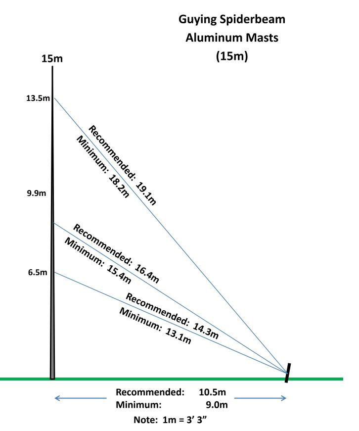
NOTE: Guy lengths shown are 2m longer than actual length to ground stake to allow for tying both ends. Cut each rope to the length shown.
