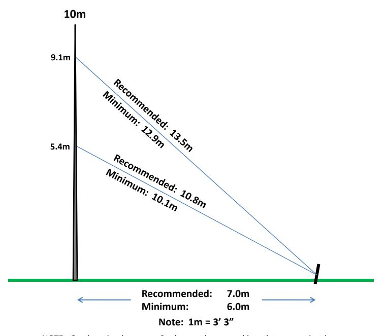
NOTE: Guy lengths shown are 2m longer than actual length to ground stake to allow for tying both ends. Cut each rope to the length shown.
