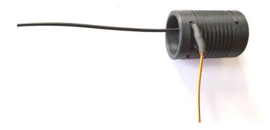
A. Now while pulling the wire tight, wind the copper wire into a coil, such that it fits snuggly into the grooves. When reaching the end of the copper wire, insert the far end of the CQ-532 wire through the hole in the coil form and pull the wire tight, such that the heat-shrink tubing is sitting in the thick groove at the end of the form and the wire does not move on the coil form.
