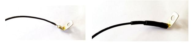
8. Repeat steps 1 through 7. Then mark the dipole legs (wires) with "DIR" and "REF".
