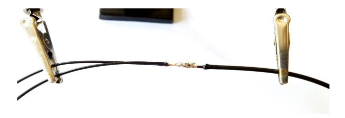
2. Slide a 50mm long piece of 3/1mm heat-shrink tubing over the splice and heat to shrink. Then slide a 30mm long piece of 6/2mm heat-shrink tubing over the 3/1mm tubing, heat to shrink. Do this for both ends of the dipole.
