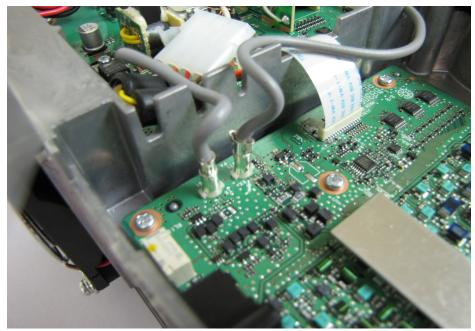
4) There are 2 cables with TMP connectors right behind where the RX7300 is to be installed in the open slot. Pull the cable out of the jack (J1701) closest to the front panel of the radio and plug it into the female TMP connector on the RX7300.
