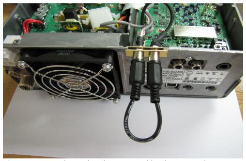
6) Slide the RX7300 mod into the place vacated by the external antenna tuner jack. There may be a little side-to-side movement of the mod kit – this is normal.
