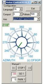
Configure the Axis to <axis1=AZ | axis2=none>.
