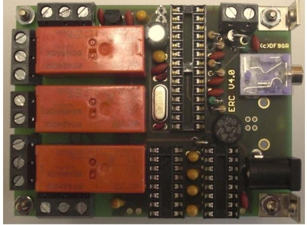
Do not place the ICs (MEGA328, MAX232 and ULN2003) into their sockets until the following testing is completed.
