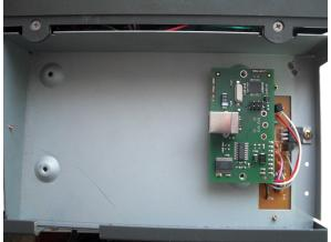
fix the ERC-Mini SDX with 2 screws M3x6 and 2 spring-washers 3.2mm as shown in the next picture
