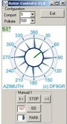
The green pointer and number show the current position of the rotator.
