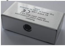
Plug the USB-cable with the USB-B-connector into the ERC-Mini.
