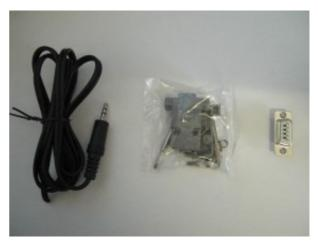
As the delivered cables differ with their colours, it has to be measured which of the inner cables is connected to what contact of the phone-jack. Alternatively to the 3-wire cable a 2-wire cable with shielding can be delivered. For this kind of cables the both shielding have to be twisted together. The shielding is representing GND.
