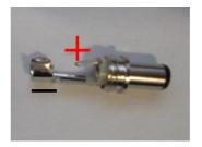
Now plug the DC-connector into J1 of the ERC-M. After connecting DC correctly, you should measure +5VDC +/-0.2V at the test-point +5V and +10 to +15VDC at test-point +12V against GND. **Disconnect the supply now.**
