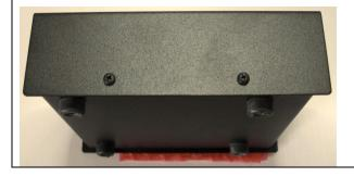
If you don't use the LAN-Option of the ERC-M, you can covert he the hole with the blind cap. Therefore cut the lamellas on one side of the cap with a knife and press the cap into the back-panel of the housing.
