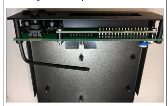
Mount the ERC-M-PCB to the housing with 4 screws M3x6.
