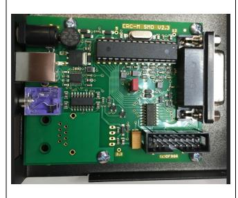
Fold the 15-pole flat-ribbon-cable as shown and put the DSUB-connectors as shown and mount the female-DSUB-connector to the back-panel of the housing with the 2 UNC-distance-bolts and 2 washers from the DSUB-mounting kit.
