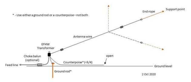
Figure 2A (top) and 2B (bottom) - Typical EFHW Installations
