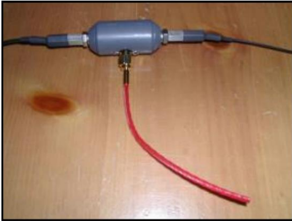
FIG. 2 SMA INSTALLED FOR 40M & 20M OPERATION
